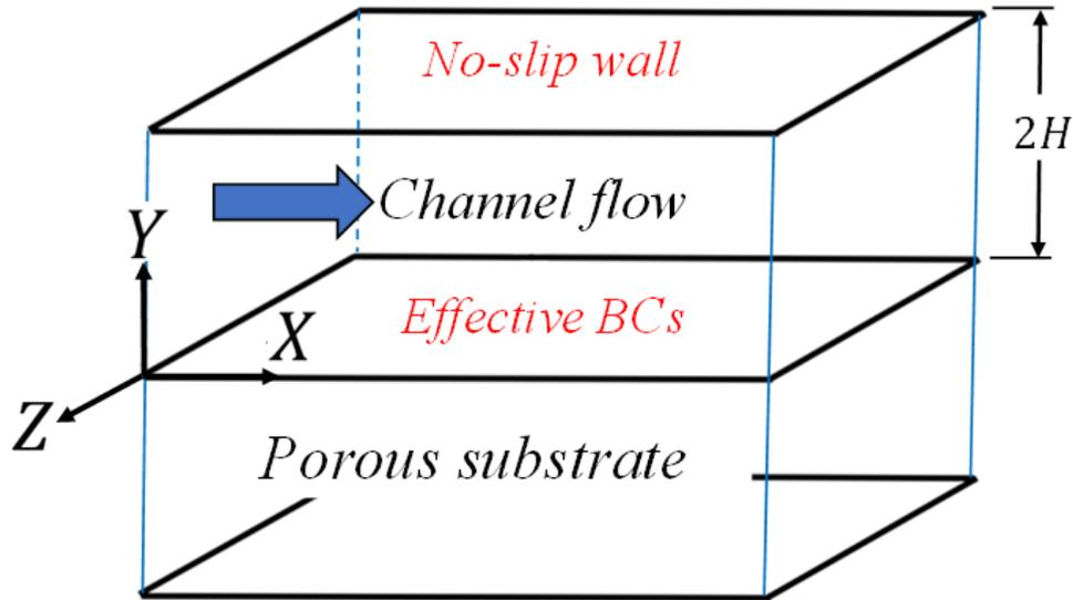
$$\left. \begin{array}{l} \tau_0: \text{Total shear stress at } Y = 0 \\ \tau_2: \text{Total shear stress at } Y = 2 \end{array} \right\} S_R = \frac{\tau_0}{\tau_2}$$
